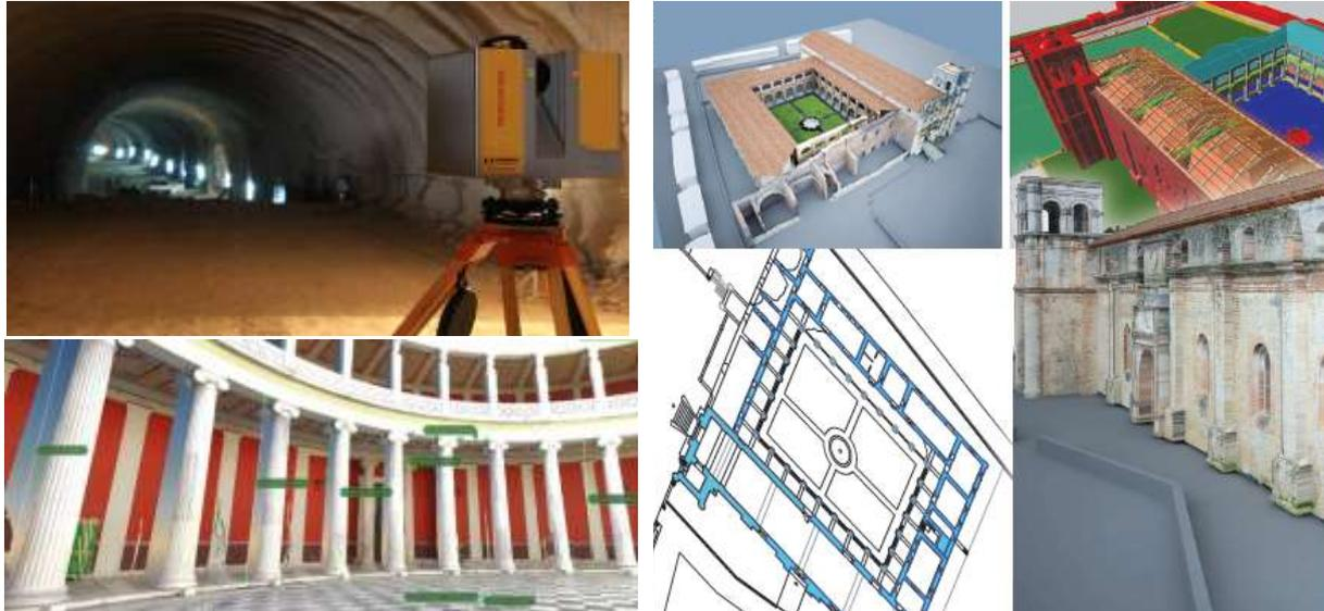
Completion of the fieldwork results in a geo-referenced point cloud which, due to its great density and its ability to bear information on the reflectivity and/or the color of each point, comes close to the term, “**virtual reality**”.
