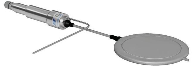
After concrete around the pressure cell has fully cured and has cooled off to the ambient temperature, the pinch tube is pinched at intervals, using a set of pliers, squeezing the fluid out of the tube into the capsule. This forces the capsule to expand until the gap is eliminated.
