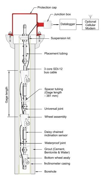
EAN-52M In-place inclinometer system with SDI-12 bus interface to SDI-12 compatible datalogger
