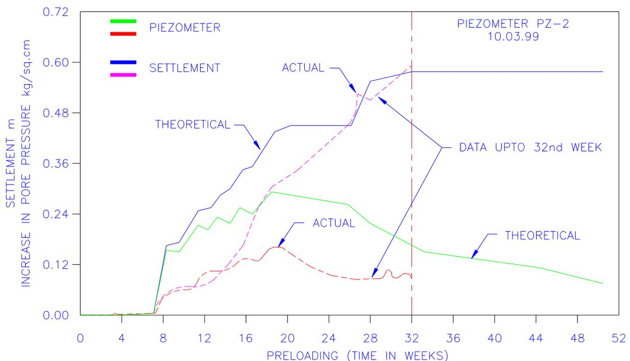
Figure 3.2: Readings of piezometer Pz-2 following expected trend
