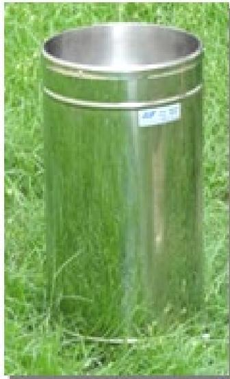
High vertical sidewalls of the model ERG-200/201 prevent splash-out of rain from the catchment thus resulting in better accuracy. Each rain gage is individually calibrated for optimum accuracy. Three adjustable legs allow the rain gage to be fastened permanently onto a platform or deck using standard fasteners.
