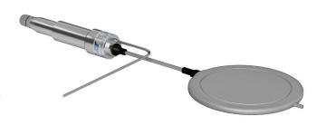
For applications in which the concrete pressure cell is embedded in concrete, a 600 mm long, fluid filled, pinch tube is welded to the sensor.
