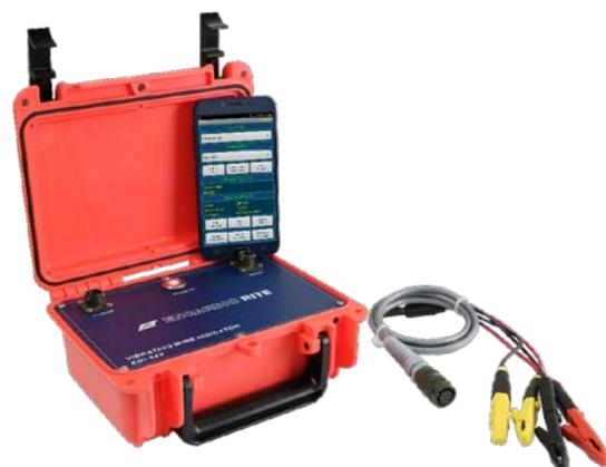
Fig 2.6 (a) – Vibrating wire indicator
