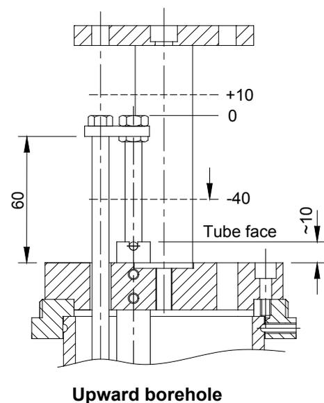
**Figure 3.4** – Procedure to set displacement sensor
