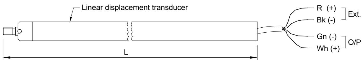
**Figure 3.1 – Potentiometric sensor**
