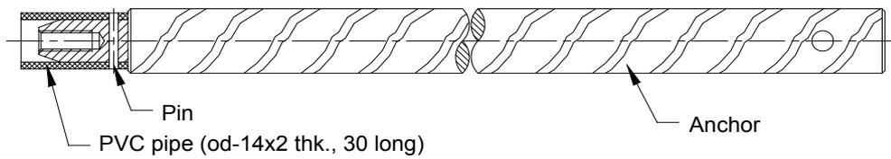
**Figure 2.7 Groutable anchor for SS connecting rods**
