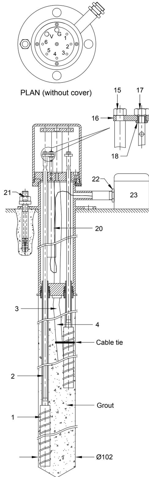
**Figure 2.4 - Six point BHE detailed assembly**
