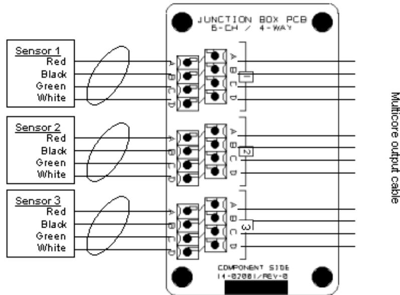
**Figure 3.5** – Junction box wiring diagram
