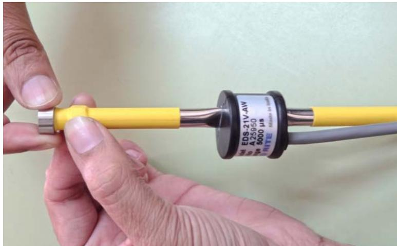
**Figure 3.2 – fine tension adjustment**
