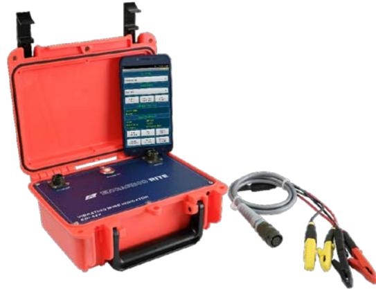
Fig 2.3 (a) – Vibrating wire indicator
