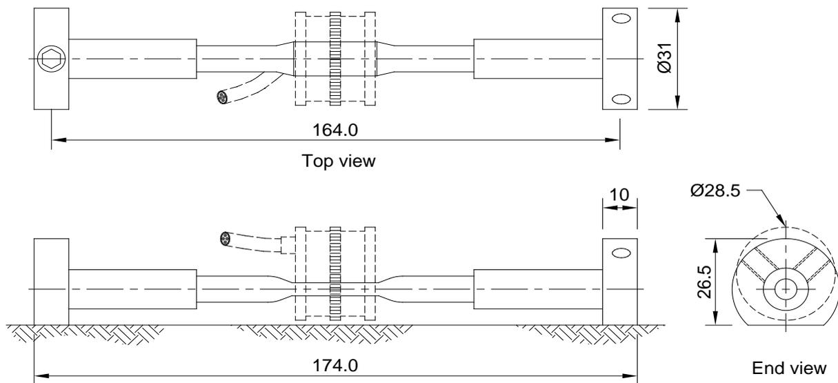
**Figure 2.1 - dimensional details with mounting blocks**
