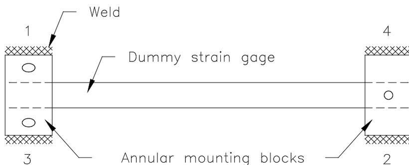
**Figure 3.3 - welding sequence**
