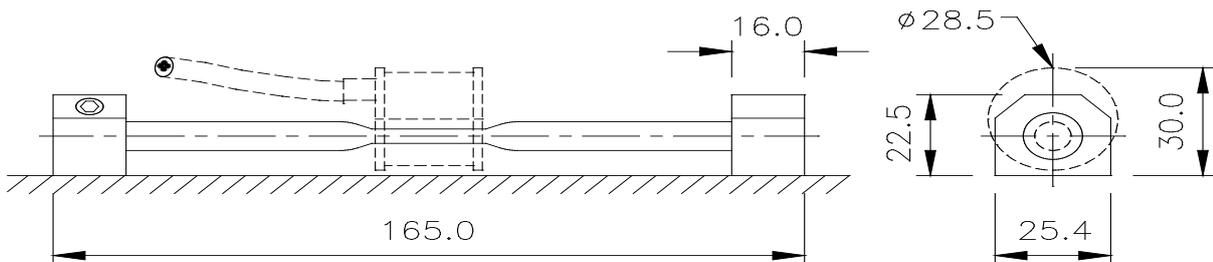
**Figure 2.2 - dimensional details with earlier mounting blocks**
