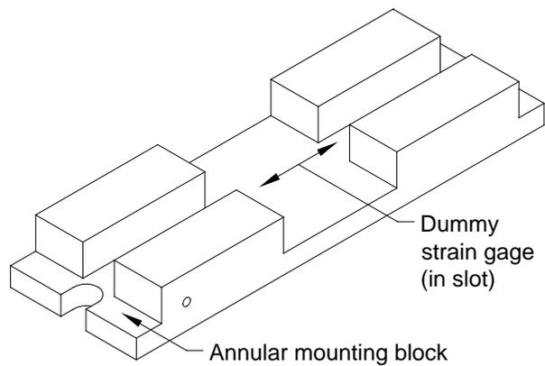
**Figure 3.2 - mounting jig**
