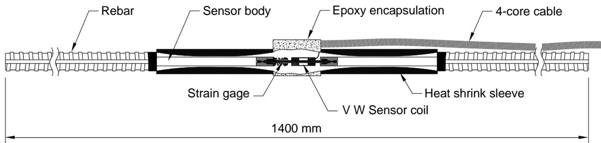
Encardio-rite model EDS-12V vibrating wire sister bar strain meter consists of a hollow bar with vw strain gage mounted co-axially inside. The hollow bar is extended on the two sides with 12 or 16 mm  $\phi$  (nominal) reinforced bars. The reinforced extensions are long enough to ensure full transfer of the strain within the concrete to the strain gage.
