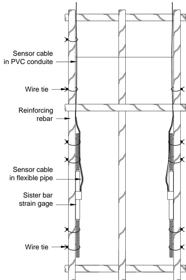
to this initial reading to determine any change in stress. The initial reading in digits along with the gage factor (from individual test certificate), constitute the calibration constants required to be fed into the EDI-54V vibrating wire indicator as set-up data for model EDS-12V.
