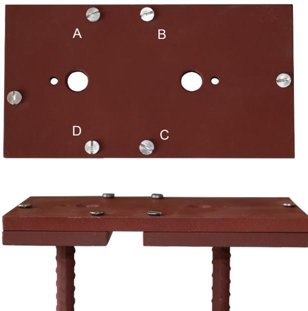
Figure 5 Grouting template
