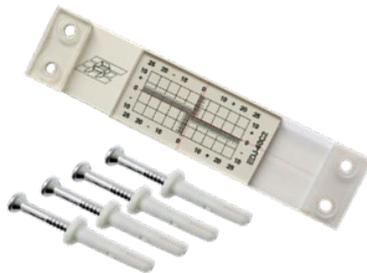
EDJ-40C2 biaxial rack meter consists of a graduated scale with a resolution of 0.5 mm and a transparent acrylic plate with a hairline cursor mark. The graduated scale and the transparent acrylic plate is assembled across the crack with expandable anchors in 5 mm diameter holes drilled to a depth of 30 mm as shown in the adjacent figure.
