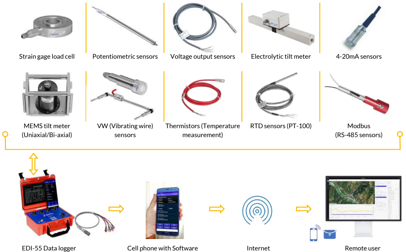
Typical schematic for multi-sensor data logging using EDI-55 data logger
