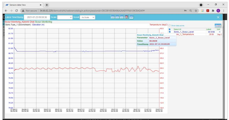
Data on Drishti from scour monitoring system (with sonar sensor) installed at a bridge in India
