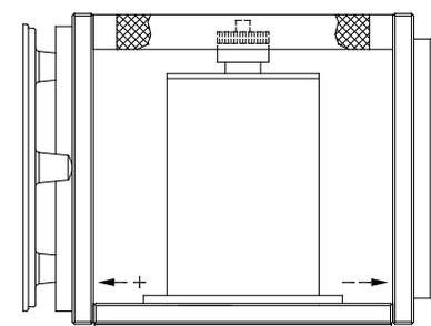
Tiltmeter placed against a vertical tilt plate
