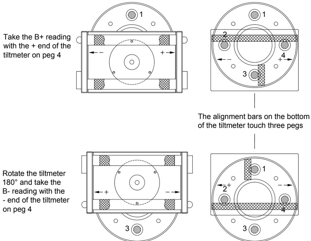
**Figure 5 taking readings in plane B**
