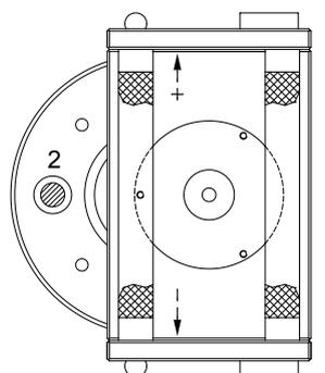
Tiltmeter placed onto a horizontal tilt plate
