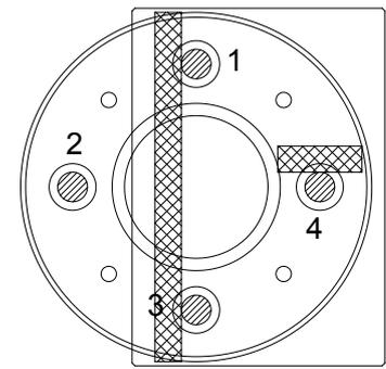
The alignment bars on the bottom of the tiltmeter touch three pegs
