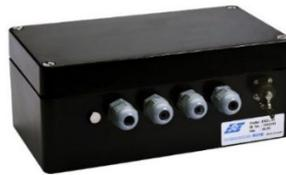
If specifically requested, the datalogger at additional cost can be programmed to process inputs from different IPI boreholes. However, this includes some limitations on the total number of sensors or IPI strings being connected, based on site conditions. Theoretically, three chains of up to 61 sensors can be connected to the datalogger. However, consult factory in case you have to install more than 60 sensors to the datalogger.
