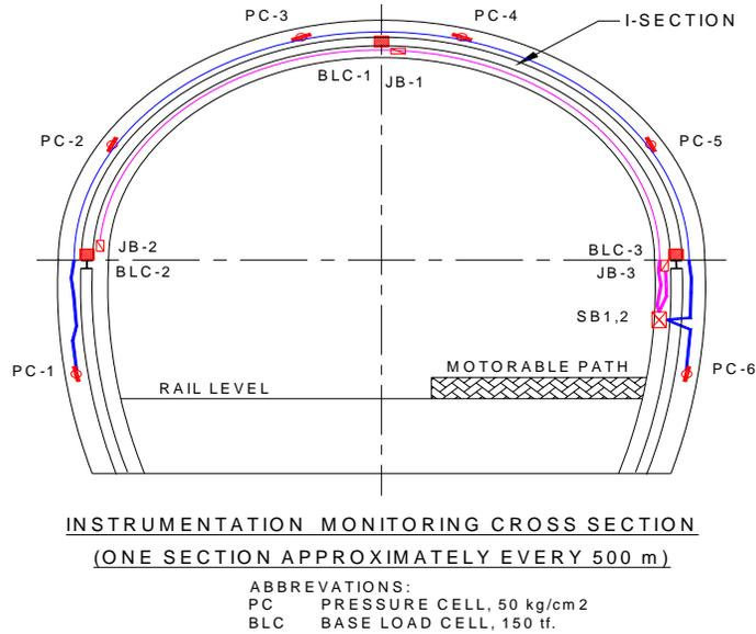
Figure 6. The section shown above, repeated every 500 m, has three compression (base) load cells of 1500 kN capacity in the I beam and six pressure cells of 5 MPa capacity in the concrete.
