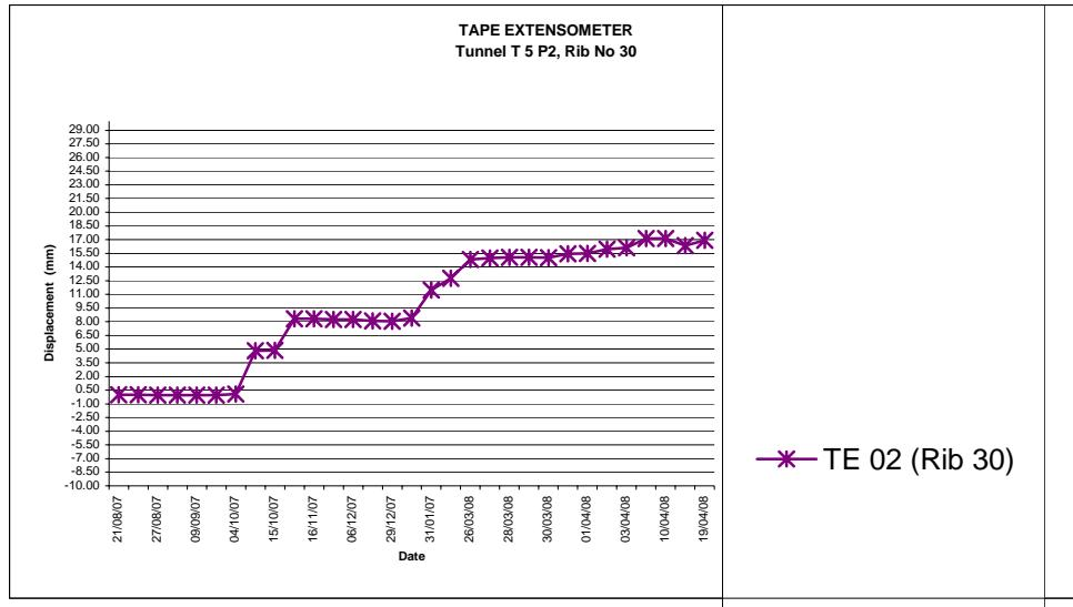
Figure 8B. Data obtained from Tape Extensometers at the same place. Immediate corrective actions were taken following this abnormal convergence.
