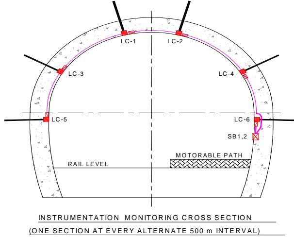
Figure 4. In this particular project, to monitor tension in the rock bolts, five centre hole load cells of 250 kN capacity are used. This section is repeated at every 500 m.
