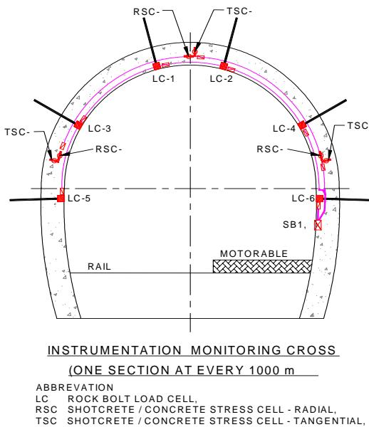
Figure 5. In this particular project, to monitor shotcrete stress, three pairs of shotcrete cells are used. Each pair has one 5 MPa cell for measuring radial and one 20 MPa cell for measuring tangential stress.
