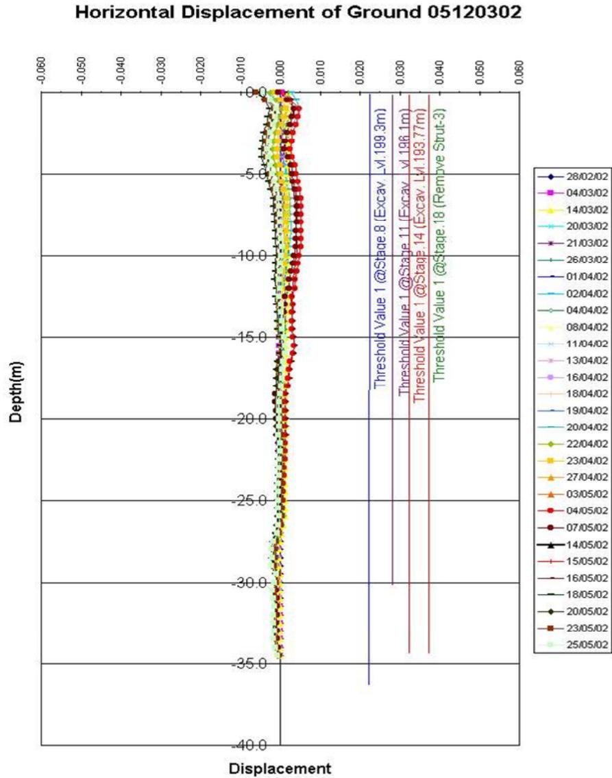
Figure 11. Typical inclinometer data inside D wall
