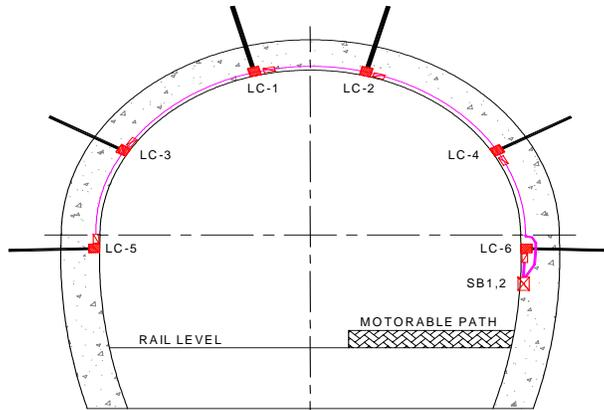
**INSTRUMENTATION MONITORING CROSS SECTION**
