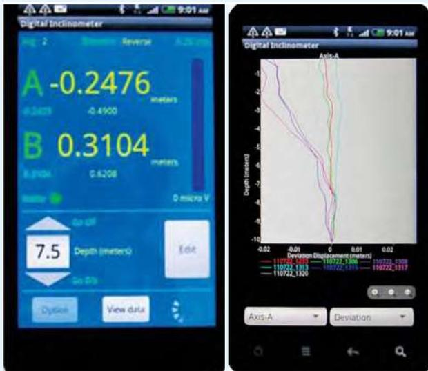
**Fig. 2 :** Mobile Phones as Readout Unit with Graphic Display
