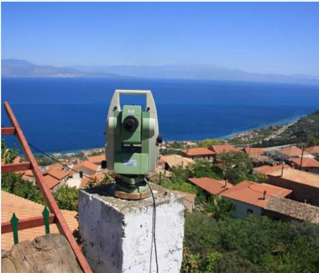
**Fig. 10 :** Monitoring by Automatic Total Station (ATS)
