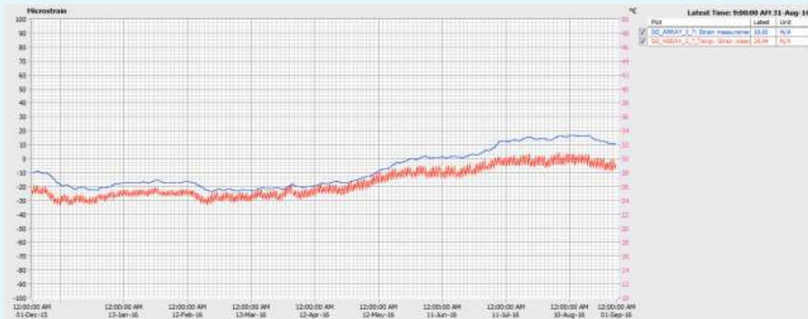
**Fig. 8 :** Shows Eight Months' Data of Variation on Strain on a Structure to Gives Important Information on Changes on Strain/Stress in The Structure with Time at that Point. The Strain Values are Affected by Changes in Temperature; so the Temperature Variation is also Plotted for Correlation on the Graph.
