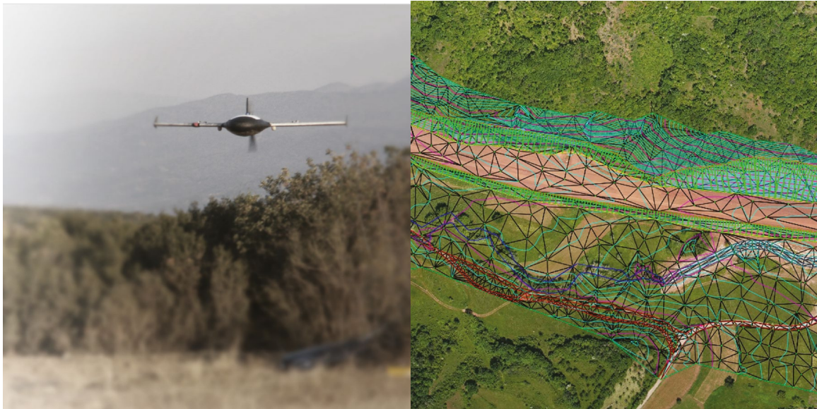
FIGURE 1: DRONE – TOPOGRAPHICAL SURVEY
