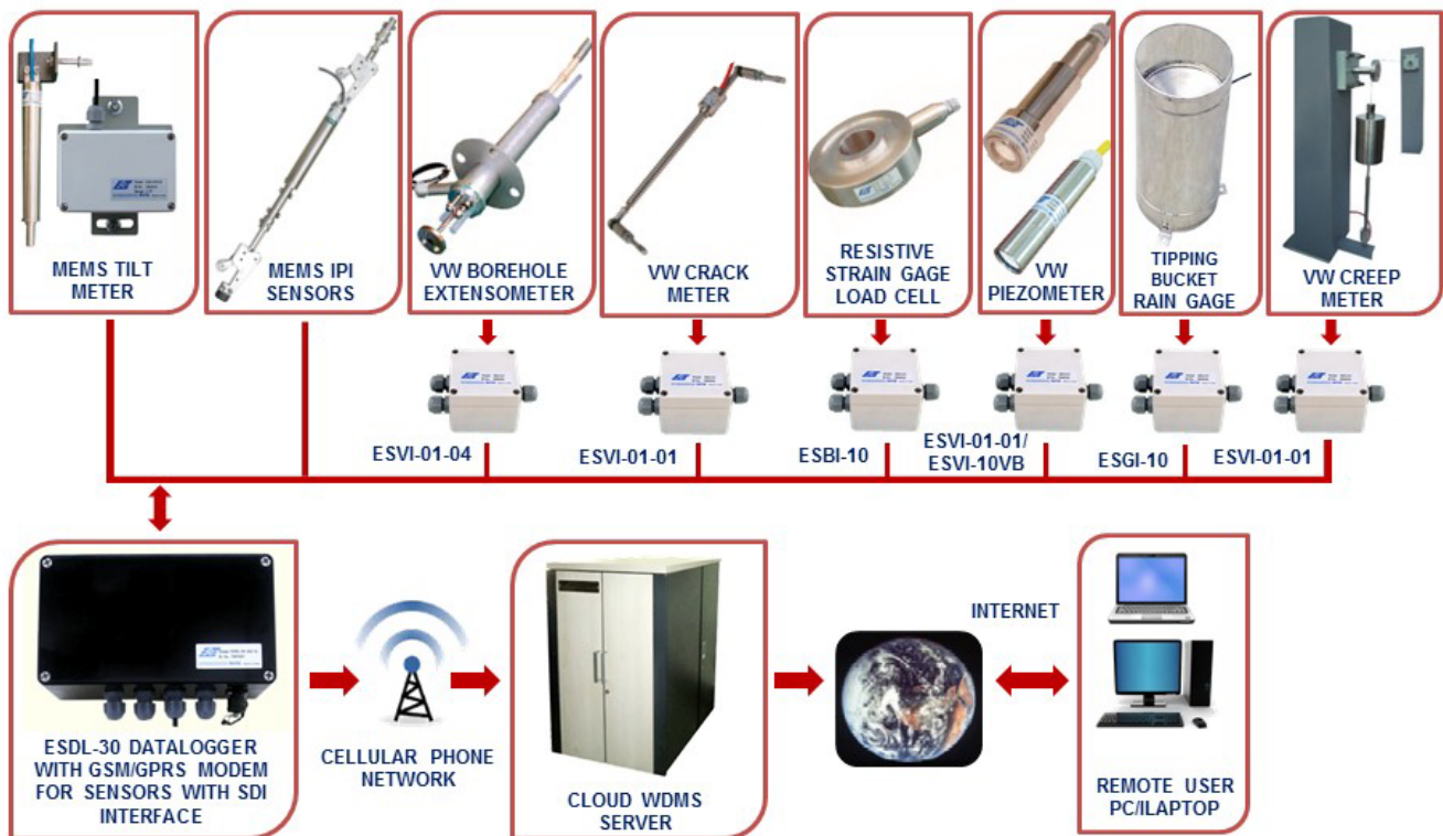
FIGURE 3: DIFFERENT SENSORS CONNECTED THROUGH SDI-12 BUS CABLE TO A DATA LOGGER WITH WEB BASED DATA MONITORING
