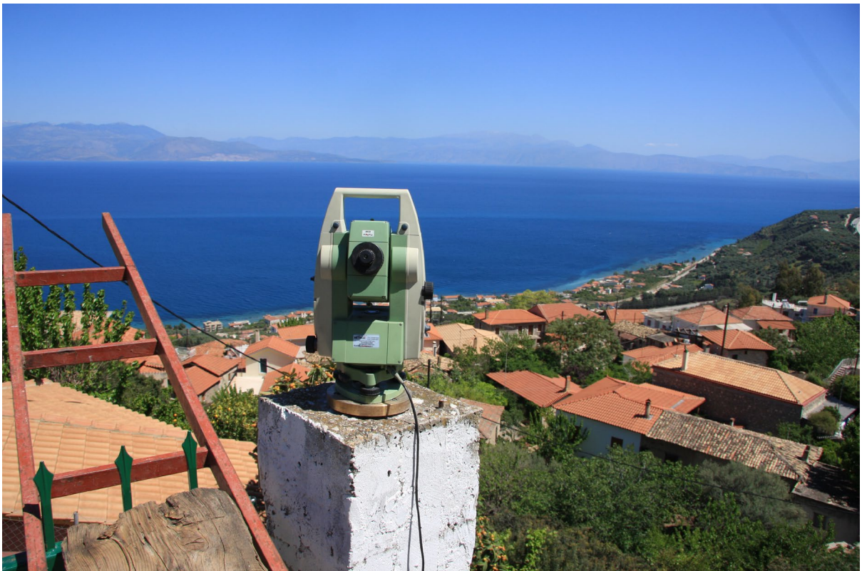
FIGURE 10 MONITORING BY AUTOMATIC TOTAL STATION (ATS)
