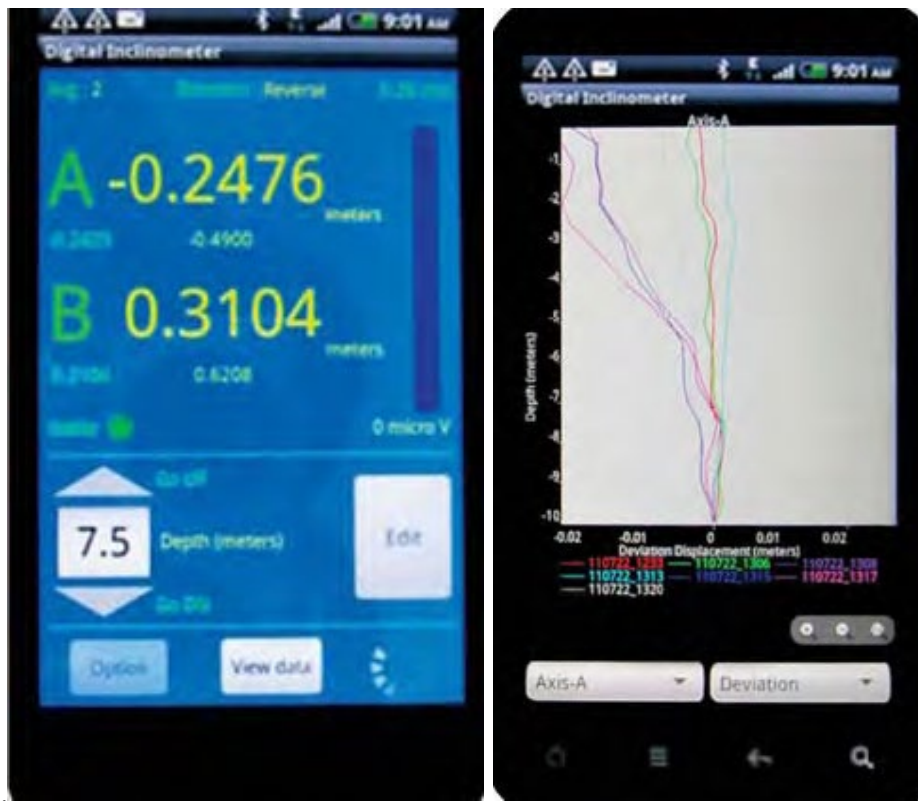
FIGURE 2: MOBILE PHONES AS READOUT UNIT WITH GRAPHIC DISPLAY
