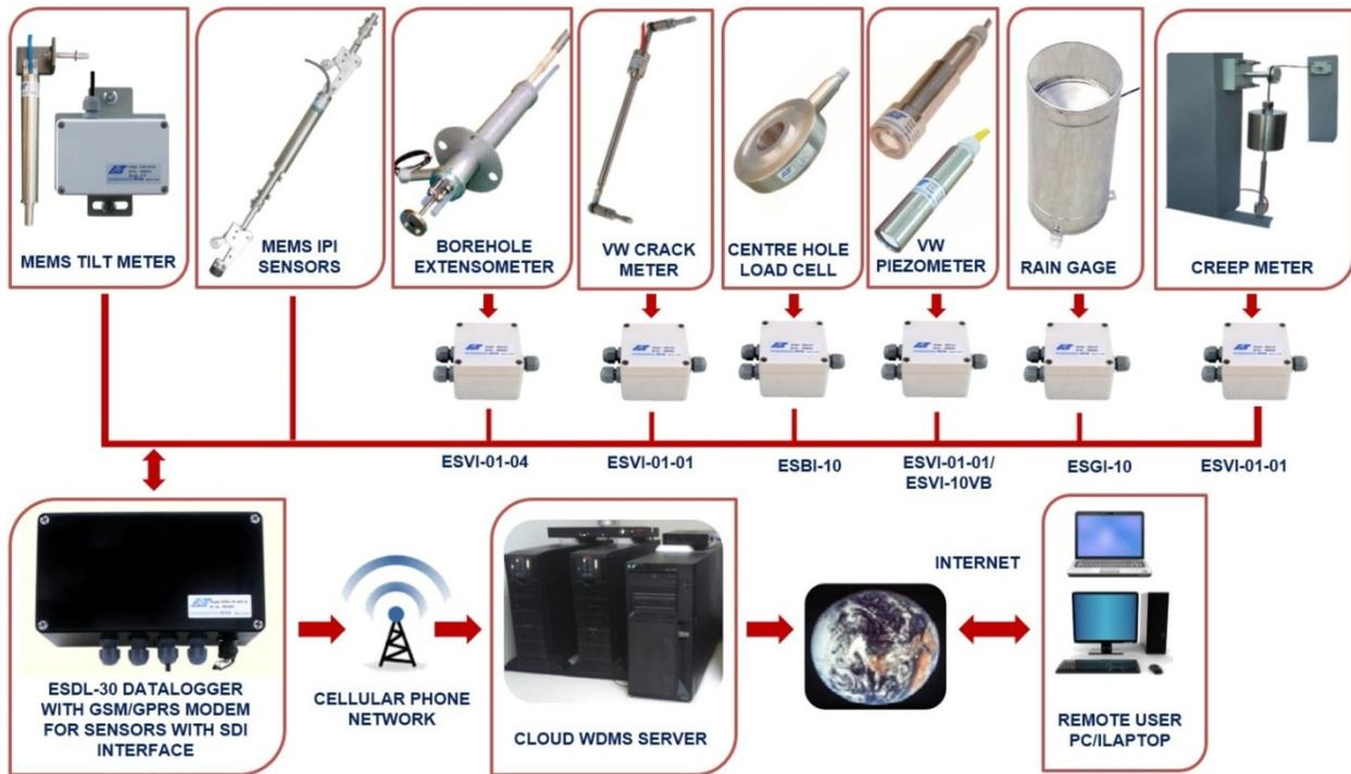
**Figure 5:** Slope stability sensors on a SDI-12 network
