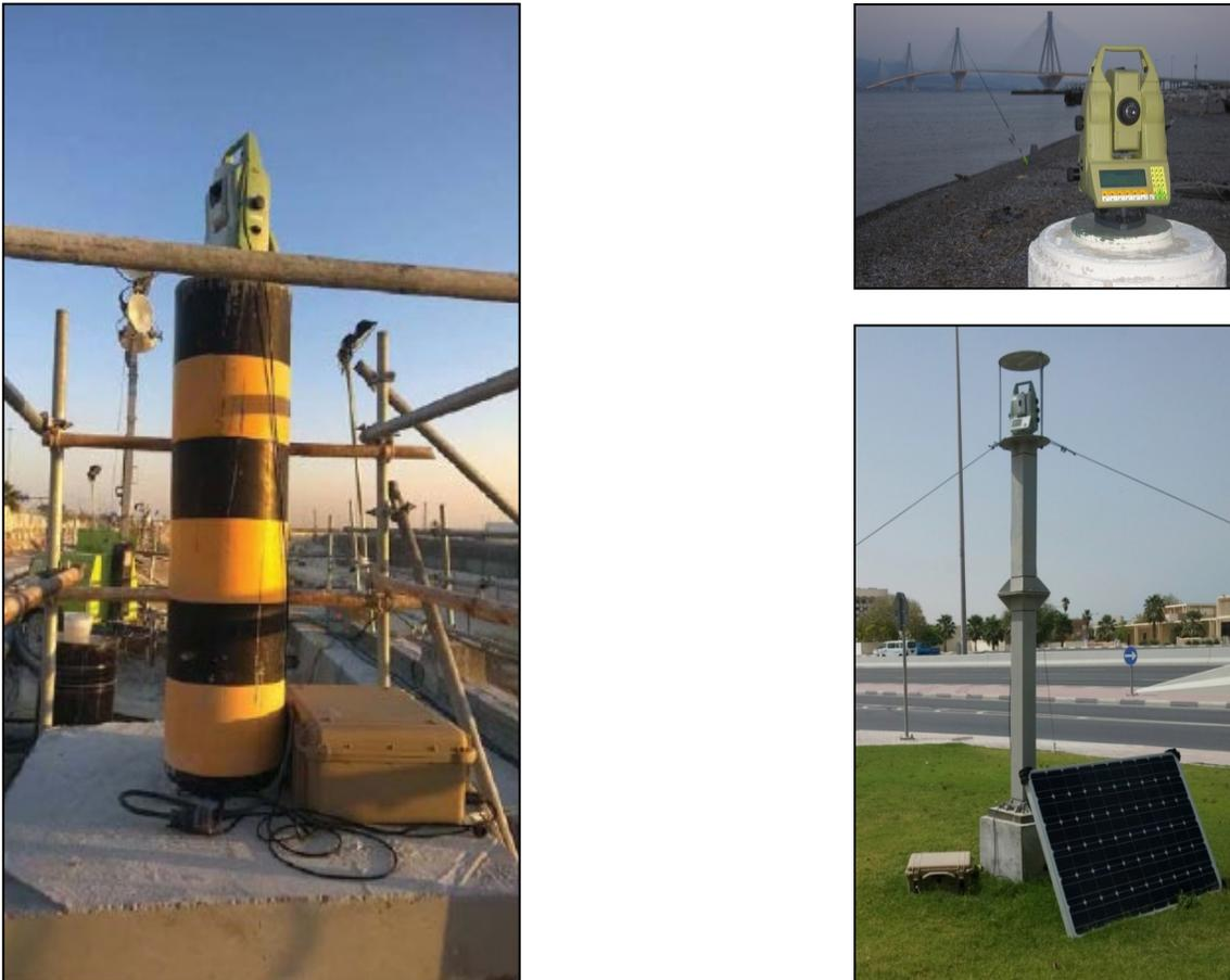
**Figure 3:** ATS with different mounting arrangements
