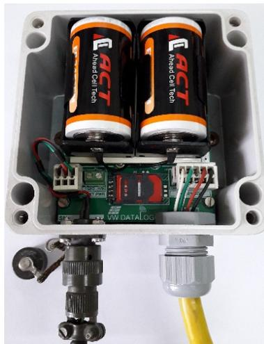
**Figure 4-2 Datalogger powered with 2 x 3.6 V Lithium Batteries**
