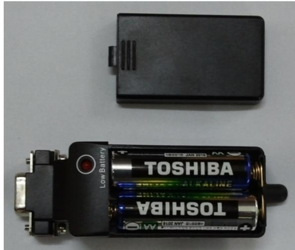
**Figure 5-5: Inserting Batteries into Battery holder**
