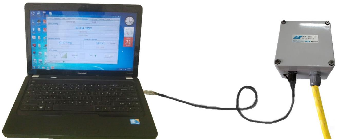
**Figure 2-3 : Connecting datalogger using interface cable**
