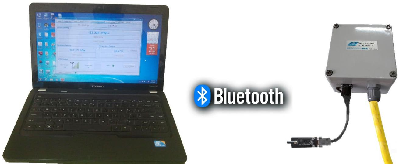
**Figure 2-5: Connecting datalogger using Bluetooth**
