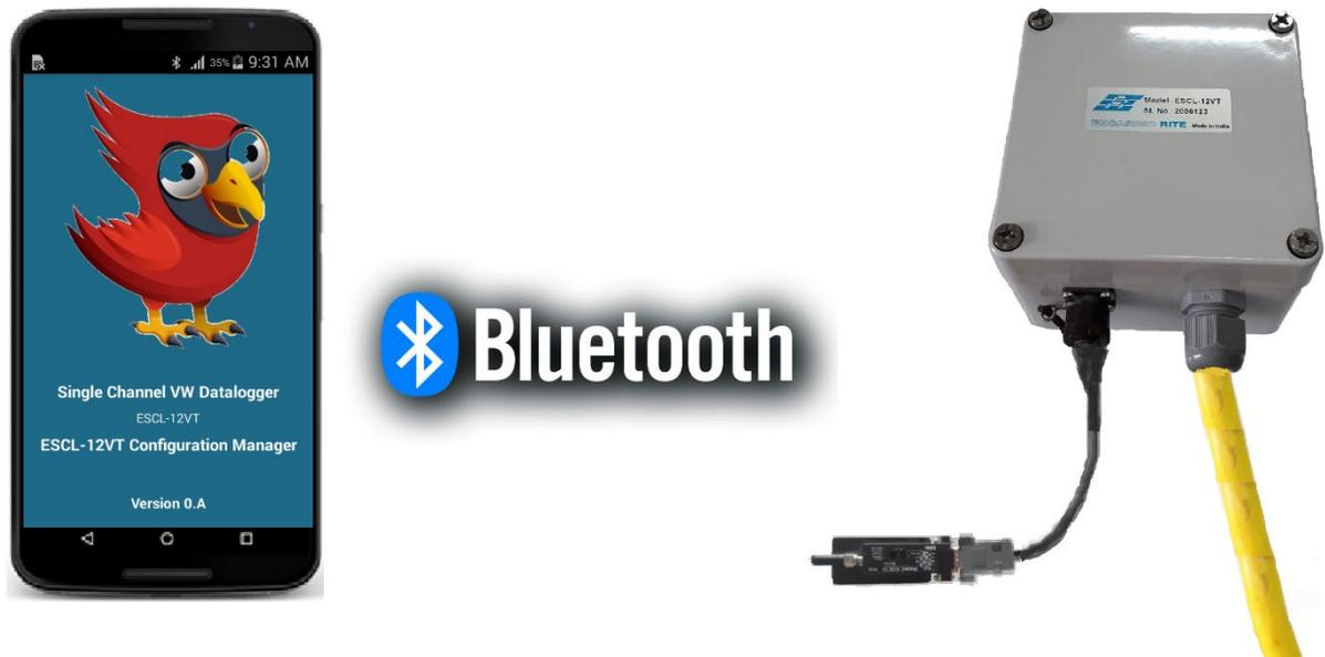
Figure 2-5: Connecting datalogger using Bluetooth
