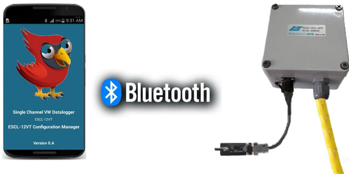
**Figure 5-8: Connecting Datalogger with Mobile Phone using Bluetooth Modem**
