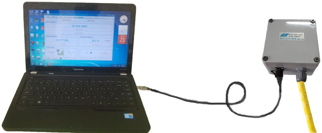
Figure 5-3: Datalogger connection using communication cable
