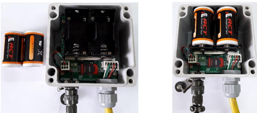
Figure 10-2: Battery replacement for Li battery option
