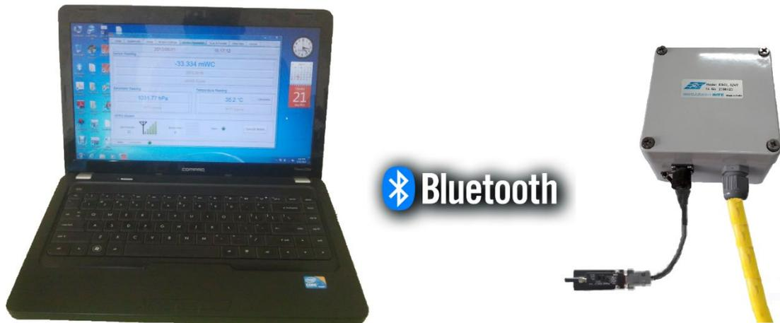
**Figure 5-7: Connecting Datalogger with Laptop using Bluetooth Modem**
