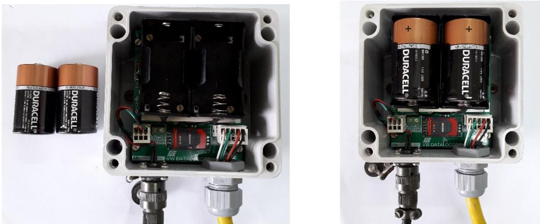
Figure 10-1: Battery replacement for Alkaline battery option
