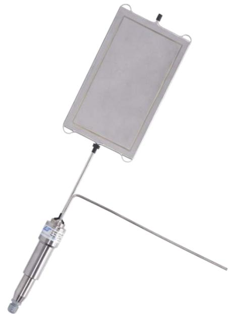
**Figure 1.1: Shotcrete Pressure Cell**
