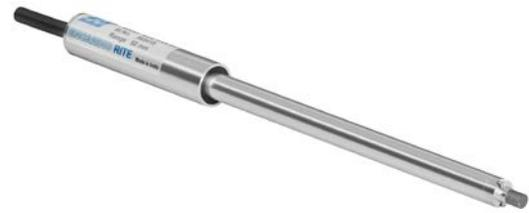
The retractable shaft of the sensor has a male thread of M6 x 12 to which the connecting rod can be attached through a link system. The sensor is provided with an integral 1 m long  $\phi$  4 mm four core cable with cores in red, black, green and white. Red and black cores are for frequency signal while green and white are for temperature monitoring through a thermistor.
