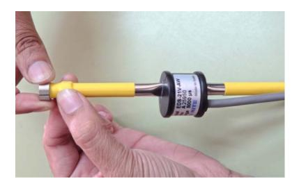
Figure 3.2 – fine tension adjustment
