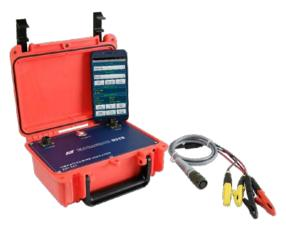
Fig 2.3 (a) - Vibrating wire indicator
