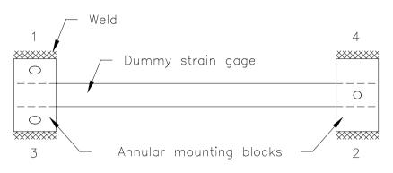
Figure 3.4 - welding sequence
