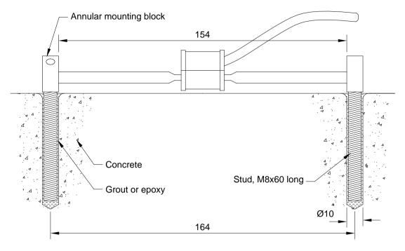
Figure 3.5 - mounting on concrete surface
