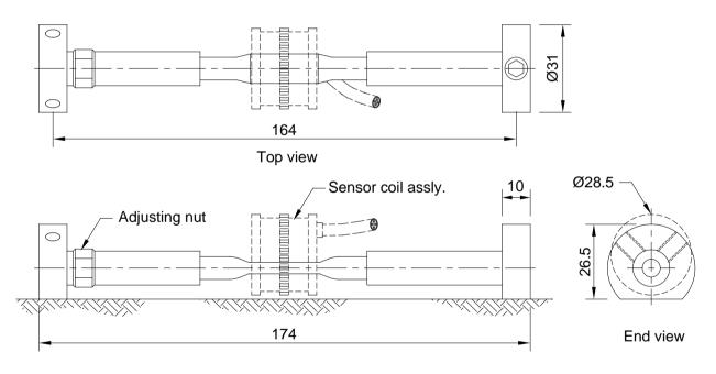
Figure 2.1 - dimensional details with mounting blocks
