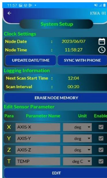
Figure 6-9 System Setup
