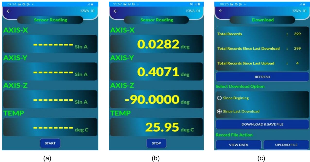
Figure 6-10 Sensor reading & Download data
