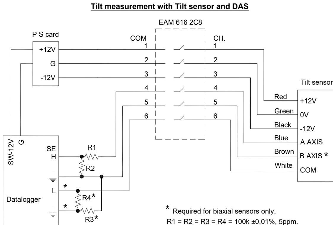
**Figure 10: Tilt meter connected to DAS**
