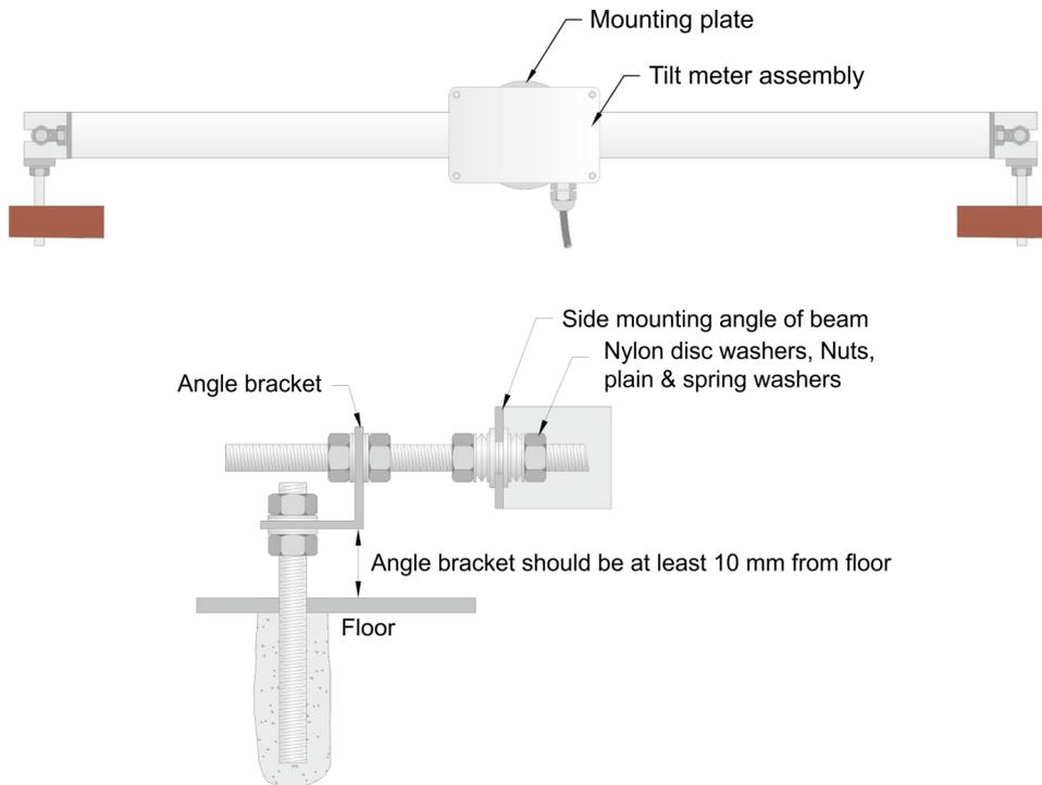
**Figure 6: Installation of EAN-91M-B sensor horizontally on the floor**
