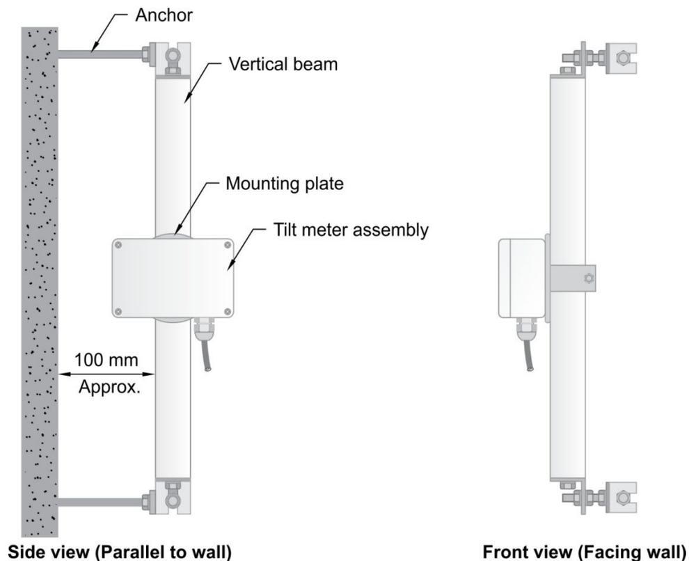
Figure 8: Installation of an individual EAN-91M-B on a vertical beam
