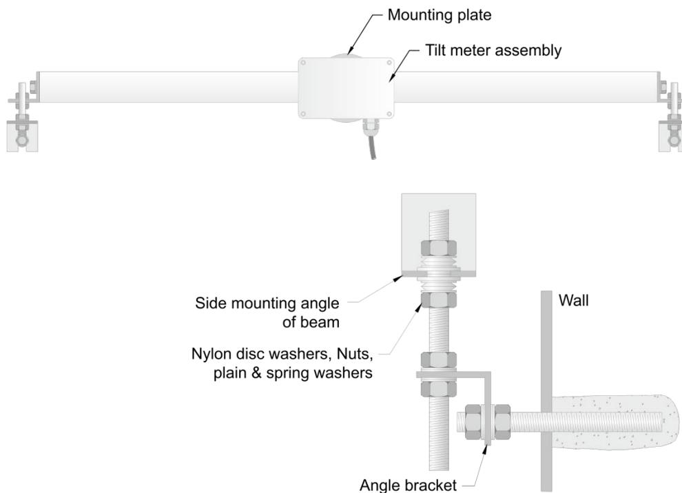
**Figure 5: Installation of the EAN-91M-B sensor horizontally on the wall**
