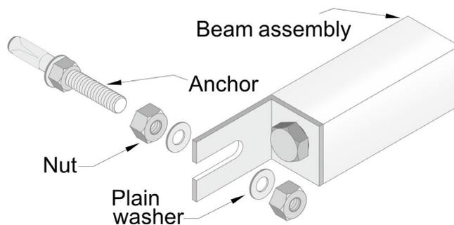
**Figure 7: Installation of an individual EAN-91M-B sensor on the wall**
