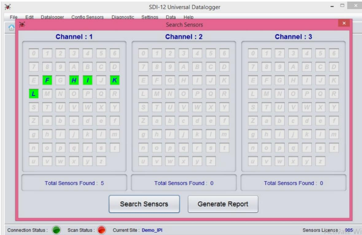
Figure 7-15 Search sensor window showing the detected sensors
