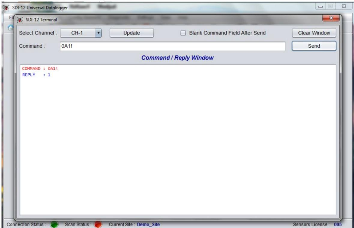
Figure 7-11 Command/Reply Window showing change in address
