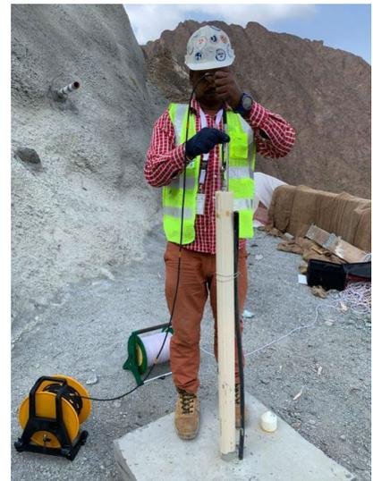
**Inclinometer readings being taken with manual probe**
