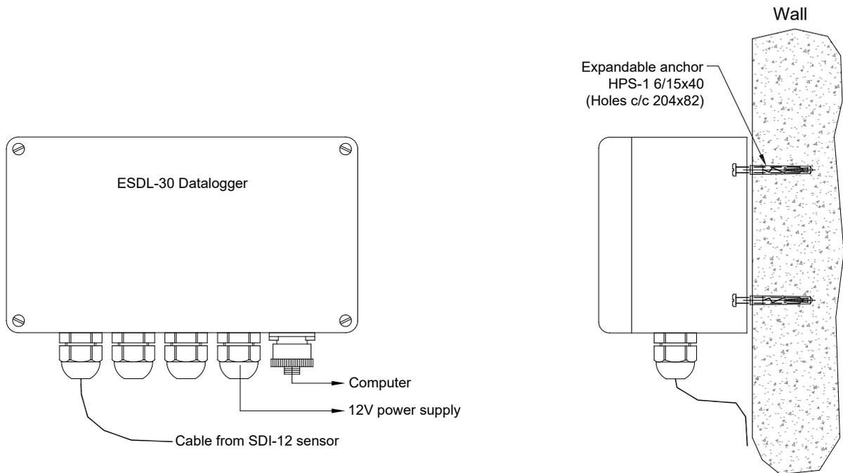
**Figure 4-1 Mounting details for ESDL-30 datalogger installation on wall/vertical surface**
