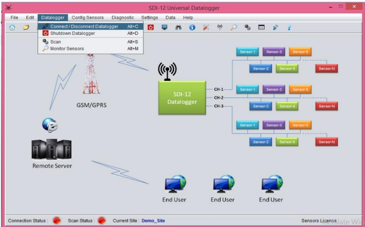
Figure 7-3 Datalogger menu of EDSL-30UNI Configuration Manger Software
