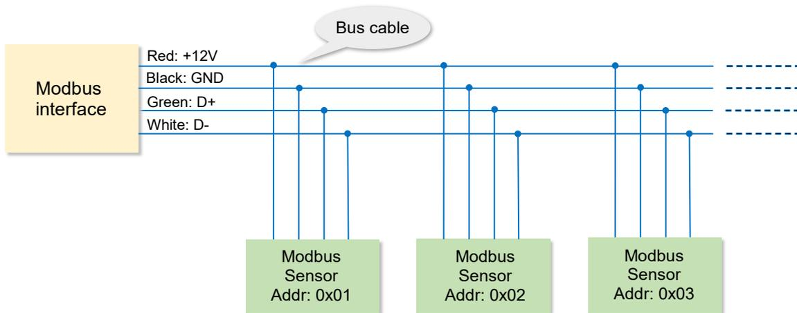
Figure 5-1 Wiring details to connect IPI with Modbus output to suitable datalogger
