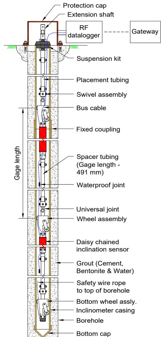
**Figure 8-1 In-place inclinometer system with RF datalogger and gateway**
