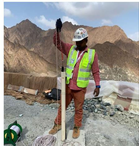
**Inclinometer gagewell being checked with dummy probe**
