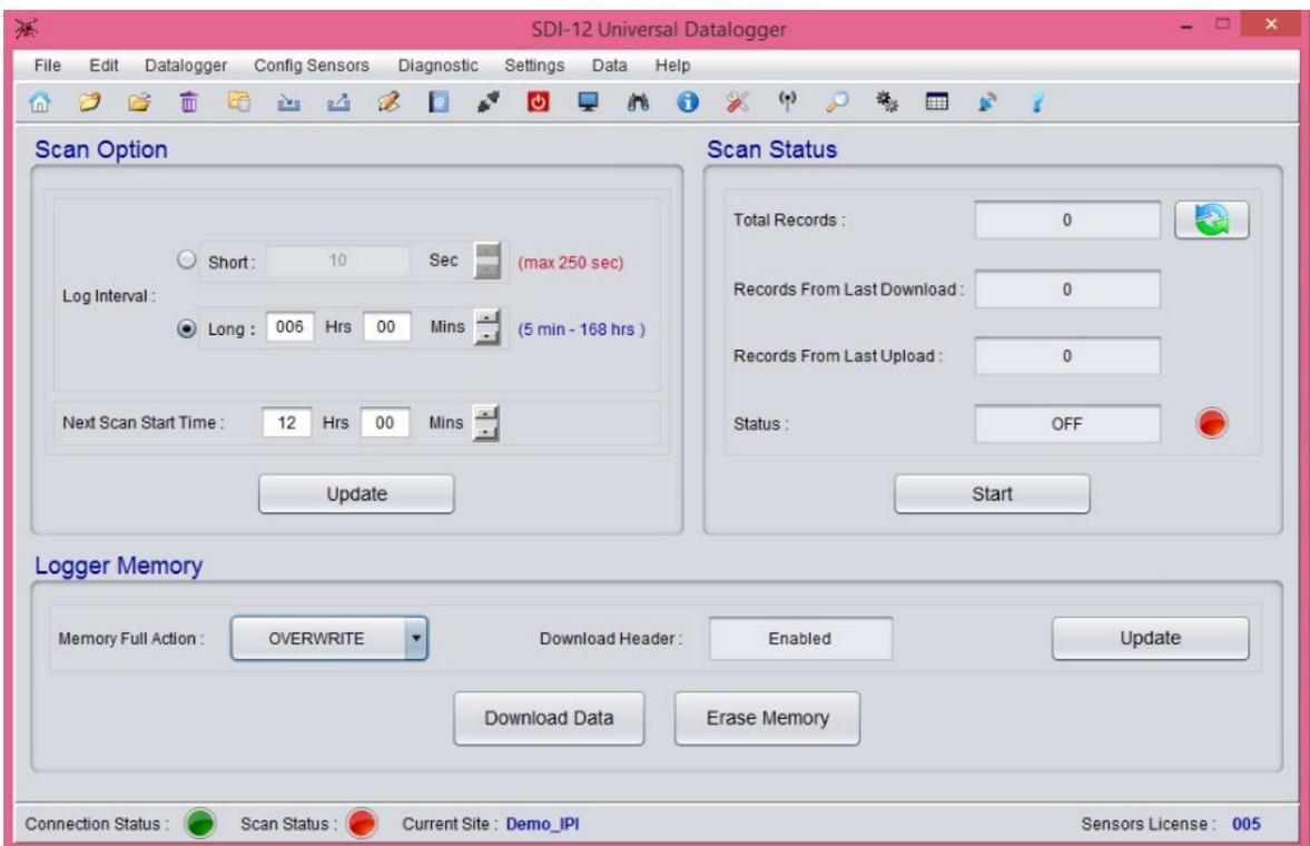
Figure 7-28 Configuring scan setting in Scan window
