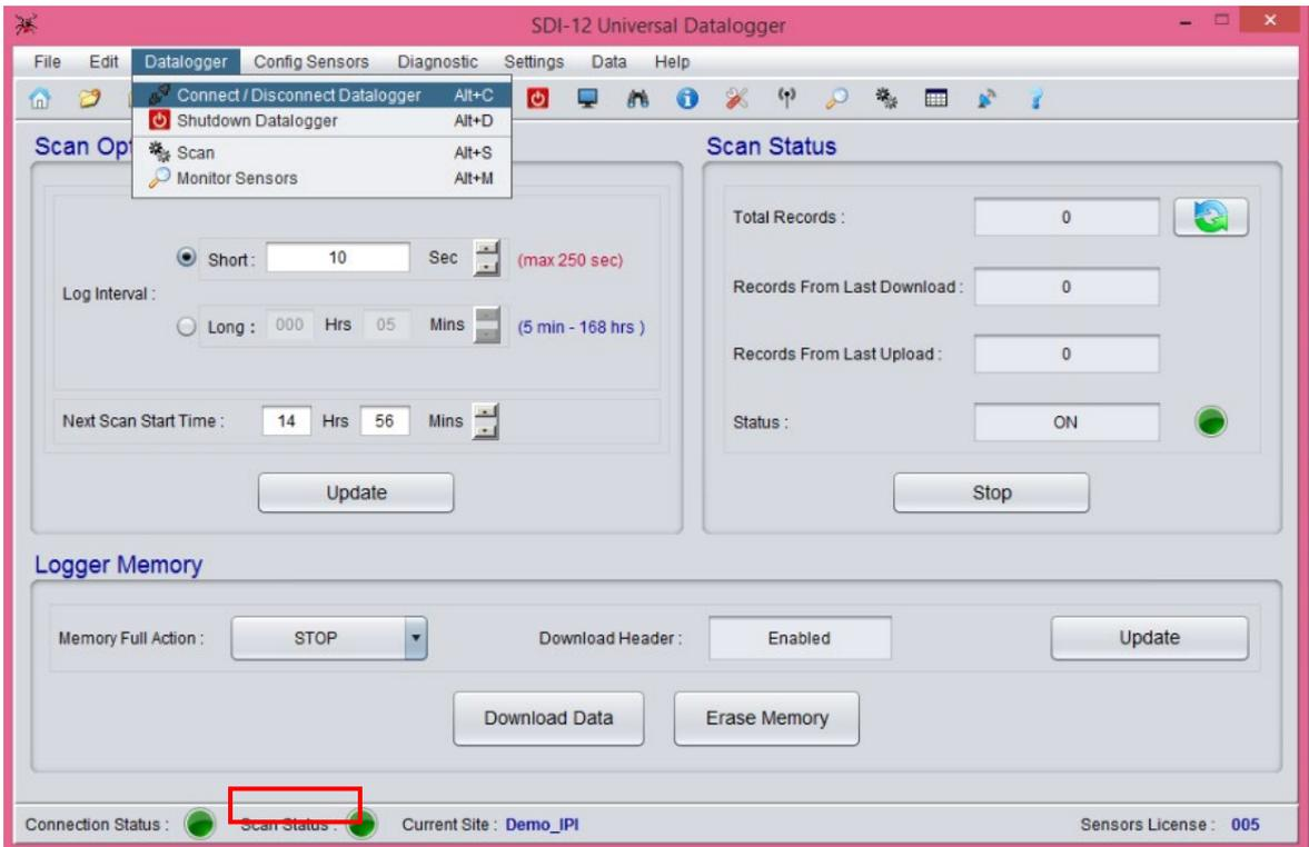
Figure 7-29 Scan status indicator in Scan window
