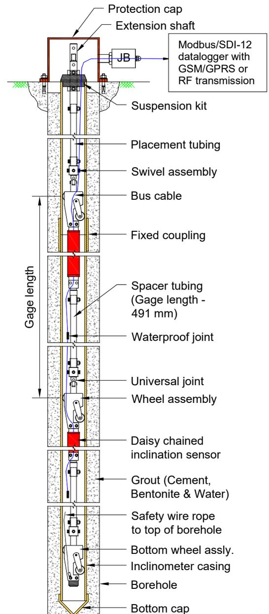
**Figure 2-1 EAN-56M In-place inclinometer system (with SDI-12 and Modbus output)**
