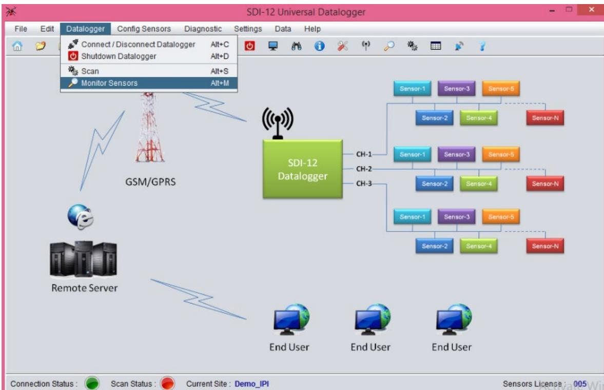
Figure 7-22 Monitor sensors option inside Datalogger menu
