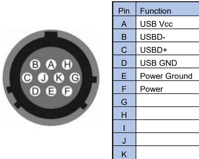
Figure 23: Power and Communications Connector
