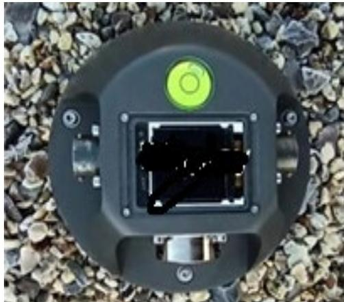
Figure 26: Top View of EADA-350F, showing LCD and Levelling Bubble
