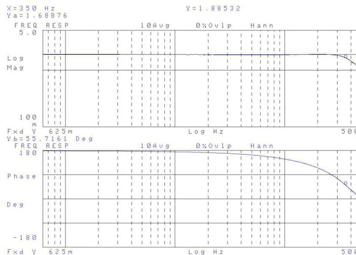
**Figure 2: EADA-350F - Typical Frequency Response to Input Calibration**
