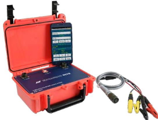
Figure 2.1: EDI-54V Vibrating wire indicator
