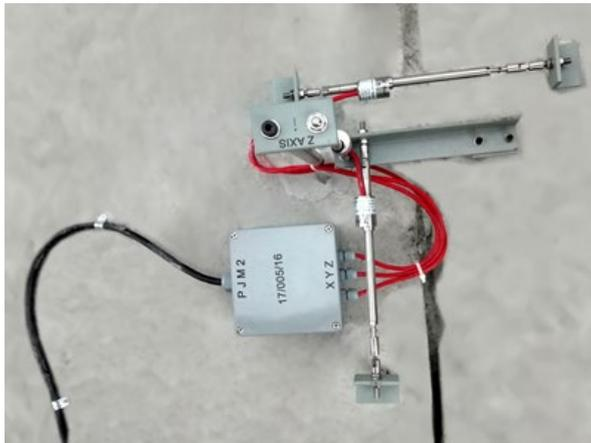
Figure 8 (a): Sensor connection with junction box – Z axis on top of the block
