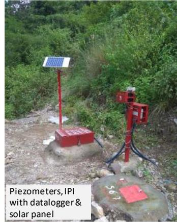
Piezometers, IPI with datalogger & solar panel
