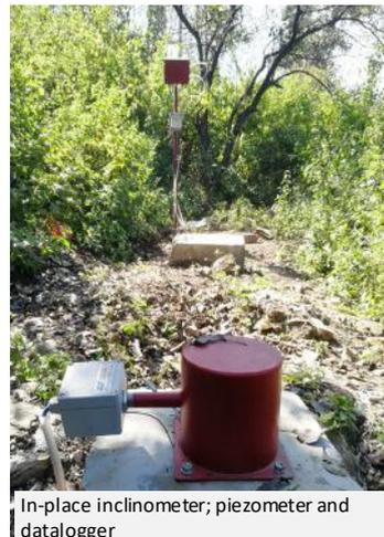
In-place inclinometer; piezometer and datalogger
