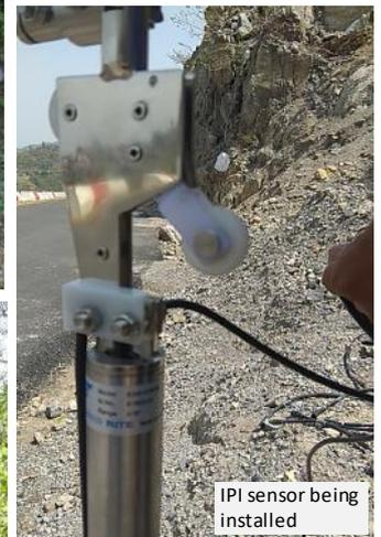
IPI sensor being installed
