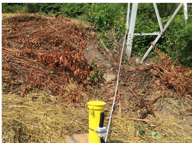
In-place inclinometer installed adjacent to the tower
