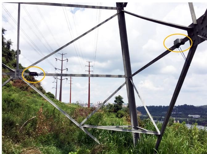
Tilt meters installed on the tower
