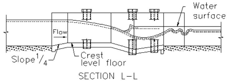
Figure 1 Parshall flume - plan and elevation
