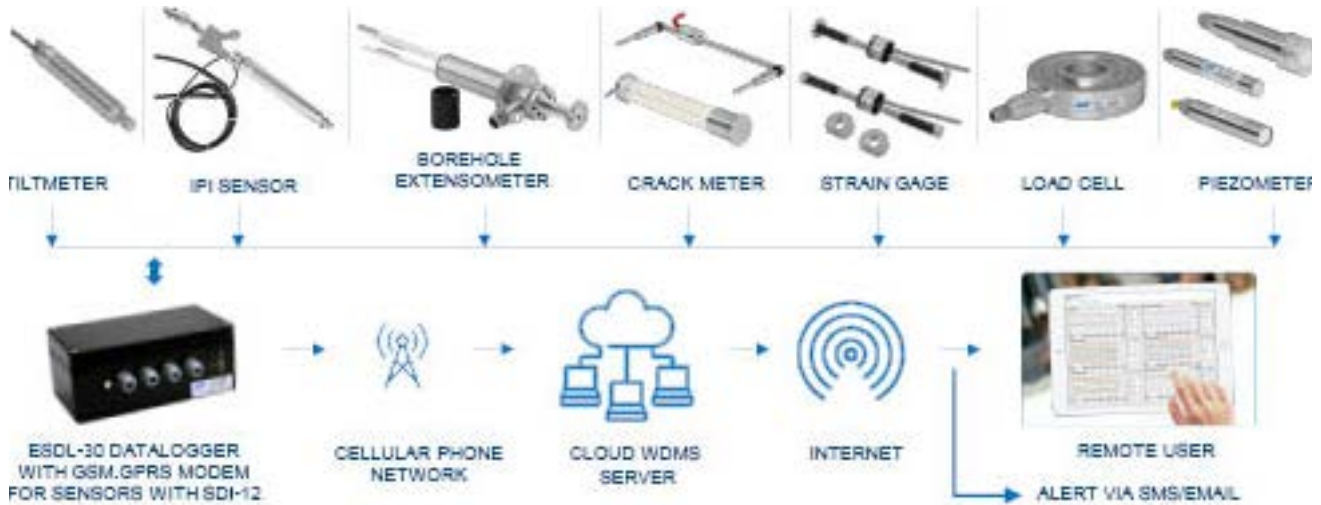
Remote real-time monitoring system with SDI-12 digital interface sensors and dataloggers
