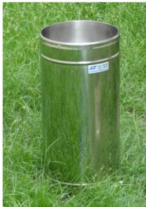
Inside each rain gage is a balanced tipping bucket mechanism with a magnet and switch assembly. Collection of rain is through a 200 mm diameter catchment through a debris filtering screen. A funnel inside the rain gage feeds collected rain water into one of the two buckets. As soon as the preset amount of water has been collected in the bucket, it tips the other way, automatically emptying the water and positioning the other bucket for collecting rainfall.
