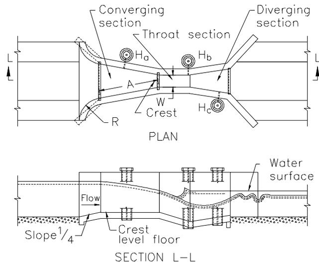
**Figure 1 Parshall flume - plan and elevation**
