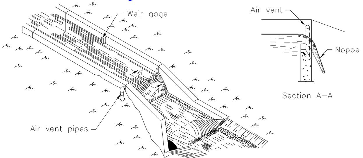
Figure 3 Standard suppressed weir
