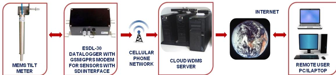
Site administrators can set two alarm limits which are generally considered as “alert level” and “evacuate level”. Other users can only view the data and alarm status but cannot make any changes.
